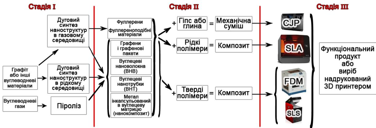
Fig. 15. Scheme of the full cycle of creating a 3D product that contains CNS, taking into account the transformation of graphite or other carbon-containing material into CNS
