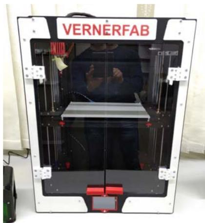
**Fig. 7.** 3D printer of FDM printing technology
