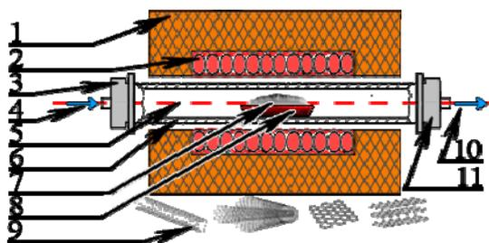
**Fig. 6.** The principle of operation of the equipment for pyrolytic synthesis of CNS: 1 – thermal insulation of the pyrolysis furnace; 2 – furnace heaters; 3 – 1st flange of the reactor with a thermocouple; 4 – directed flow of carbon-containing gases; 5 – axis of the reactor; 6 – quartz reactor; 7 – catalyst layer; 8 – lining; 9 – synthesized CNS; 10 – directed flow of gases for disposal; 11 – the 2nd flange of the reactor
