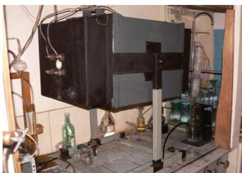
**Fig. 5.** Photo of the equipment for pyrolytic synthesis of CNS
