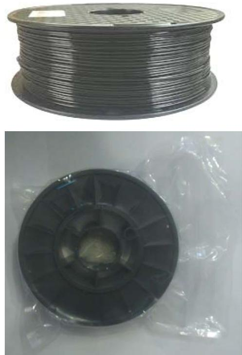
**Fig. 18.** Composite threads (hard polymer–CNS) in the bays
